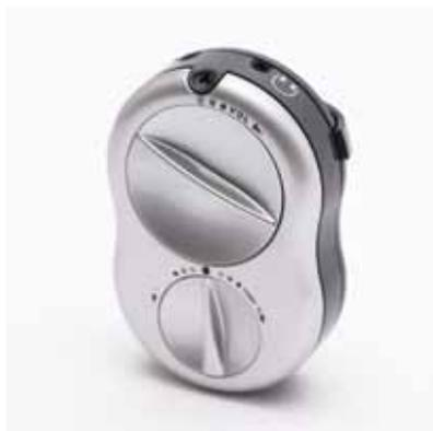
'Personal Listeners' are devices which can help someone with a hearing impairment to hear conversations. The Crescendo comes with a tie-clip microphone and a 4 metre lead so that it can be connected to the TV, radio or hi-fi. It also has a built-in microphone. It is available with either stetoclips for non-hearing aid users or a neckloop for those with a hearing aid fitted with a T switch. The unit has a large twist control making it ideal for anyone with dexterity difficulties.
